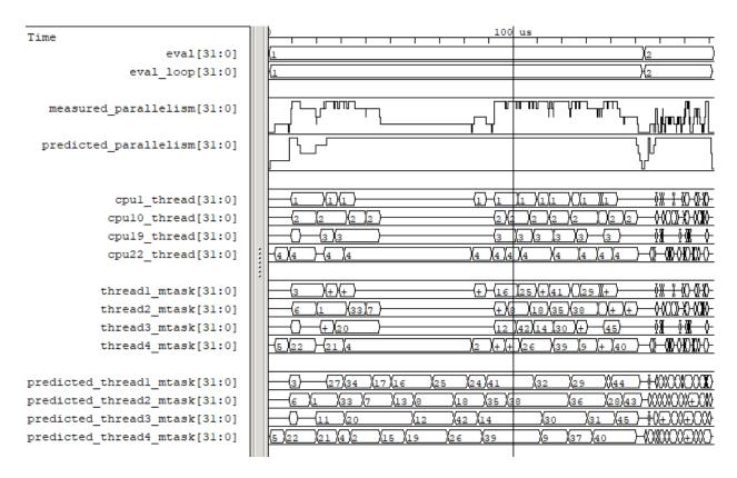
Fig. 12.1: Example verilator\_gantt output, as viewed with GTKWave.
