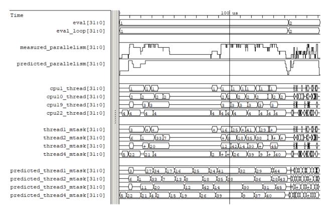
Fig. 7.1: Example verilator\_gantt output, as viewed with GTKWave. The measured\_parallelism shows the number of CPUs being used at a given moment. The cpu\_thread section shows which thread is executing on each physical CPU. The thread\_mtask section shows which macro-task is running on a given thread.
